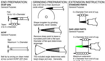
Remove sharp point to leave a truncated point with a flat spot. Diameter of flat spot determines The included angle determines weld bead shape and size. Generally, slowly increase current to form as the included angle increases. the desired ball diameter. penetration increases and bead
