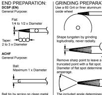
Shape tungsten by grinding Remove sharp point to leave a truncated point with a flat spot. Diameter of flat spot determines The included angle determines weld bead shape and size. Generally, as the included angle increases. penetration increases and bead
